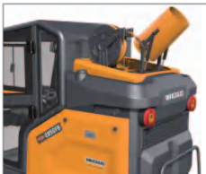
雾炮和高压冲洗
